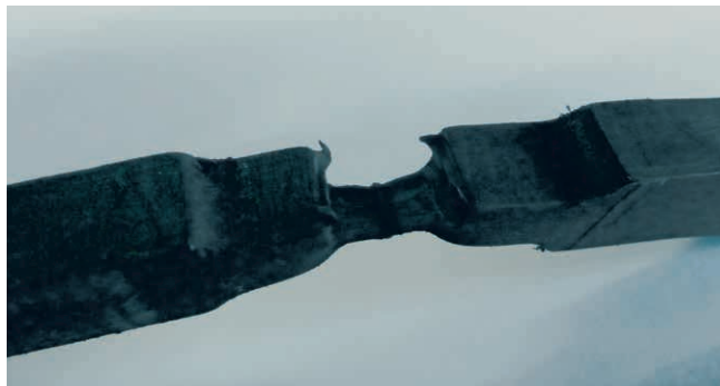
Sample following creep stress in weld zone.
