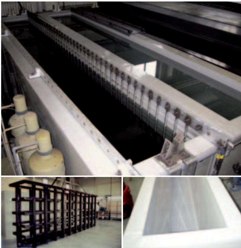
The view of the electroplating tanks shows the "loose-shirt lining" system, with SIMONA® PP-DWU outside and SIMONA® PVDF inside. Bottom left: View of the steel cross ribbing.
